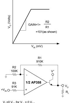
$V_{O}$ =0  $V_{DC}$  for  $V_{IN}$  = 0  $V_{DC}$ A<sub>V</sub> =10
